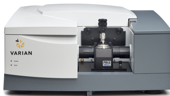
Figure 2. Varian 640-IR spectrometer with ATR fitted
