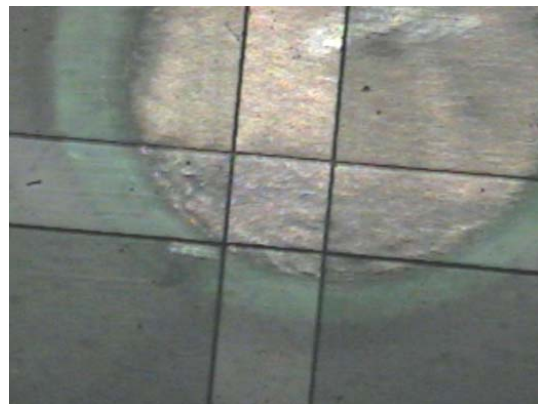
Figure 1. Visible image of Sample 1 including ViewThru apertures of the Varian microscope. Analysis area is represented by the square box formed by the four aperture blades in the image centre.
