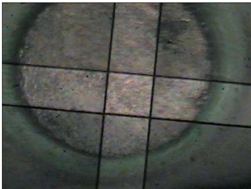
Figure 3. The visible image of Sample 2 including ViewThru apertures of the Varian microscope. Analysis area is represented by the square box formed by the four aperture blades in the image centre.
